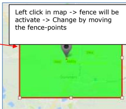
Pulling the fence sufficiently large to ensure 1x positioning inside ("leaving the area" see below) of the fence. Otherwise no tripping possible when crossing the fence
